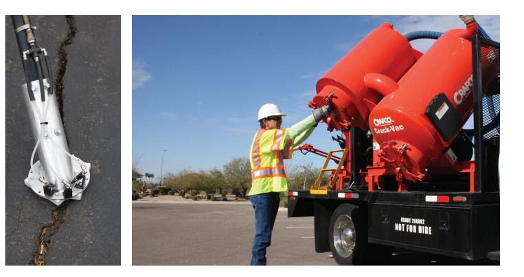
Air quality is our most important concern. The Crafco Crack-Vac cleans pavement cracks and maintains a clean environment while preserving work and public safety. The Crack-Vac boom extends in front of the truck cab keeping the worker out of traffic areas. With a filter system that contains particle matter down to ten microns (PM 10), the Crack-Vac complies with the strict air quality standards in effect today.
