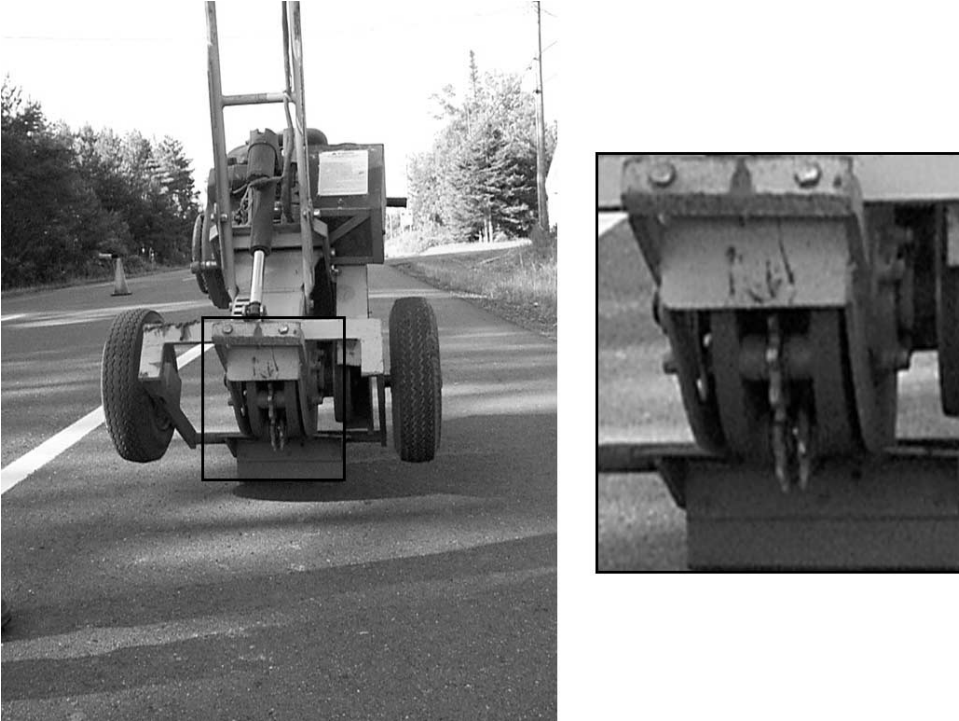
Figure 3.1 - Rotary impact router with close-up of blade
