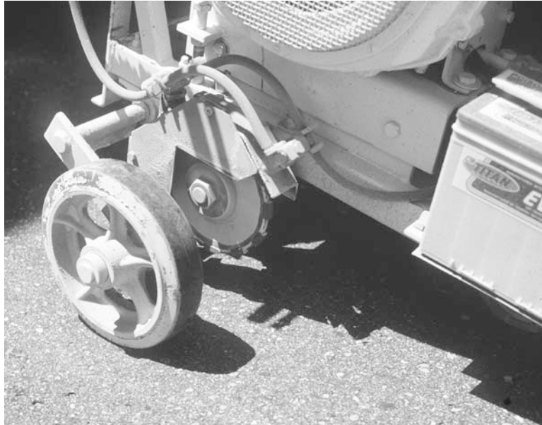
Figure 3.3 - Close-up of diamond saw blade
