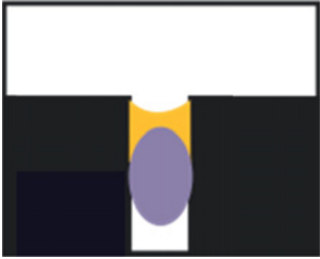
Graphic 2-3. Backer rod (shown as an ellipse) as a bond breaker (21).
