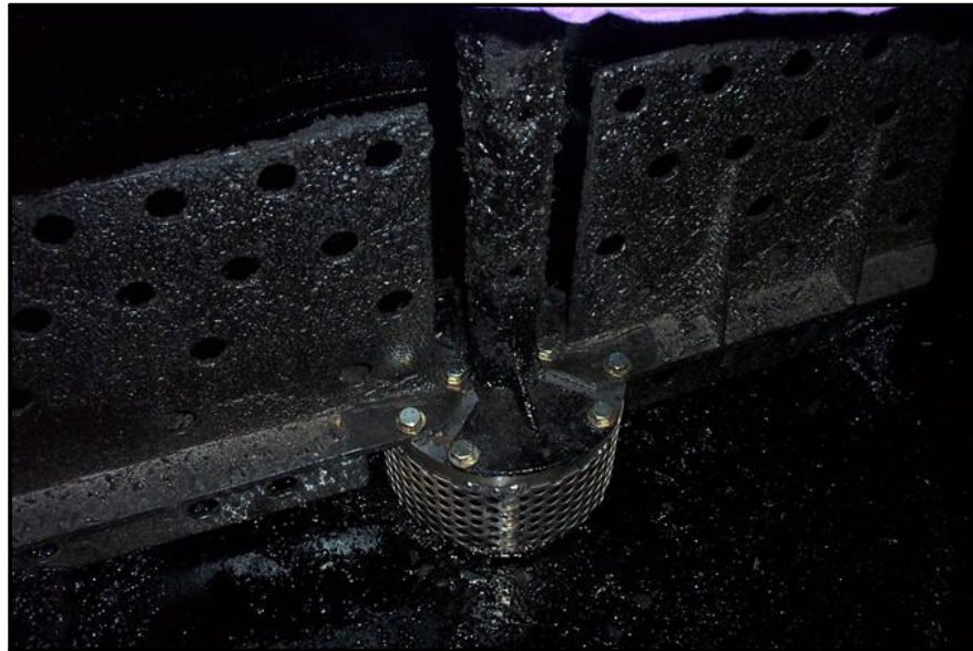
Fig. 6-10 Agitator Shaft and Paddles Mounting
