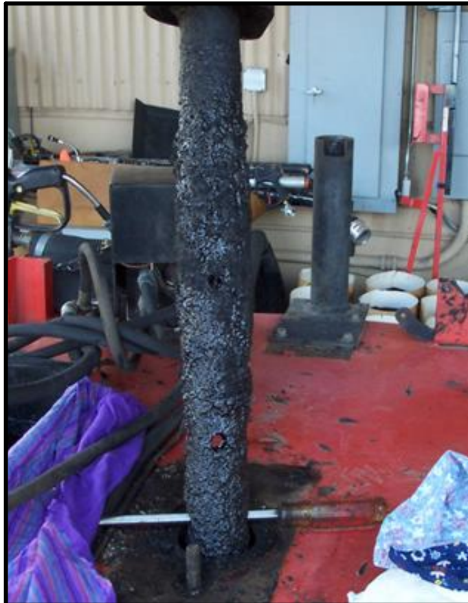
Fig. 6-5 Supporting the Agitator Away from the Material Pump
