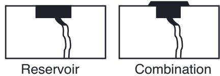
*Figure 7. Crack Sealing with Routing Common Configurations*
